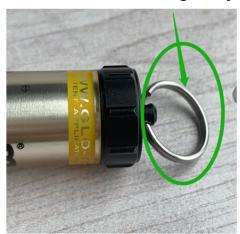
If this RING is not twisted tightly, then the light will have the "chance" of turning ON/OFF or switch the Mode during your dive.
